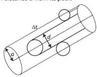
In  $\Delta t$  time, it will collide with all the molecules in the cylinder of volume  $\pi d^2 v \Delta t$ . Let n be the number of molecules per unit volume
